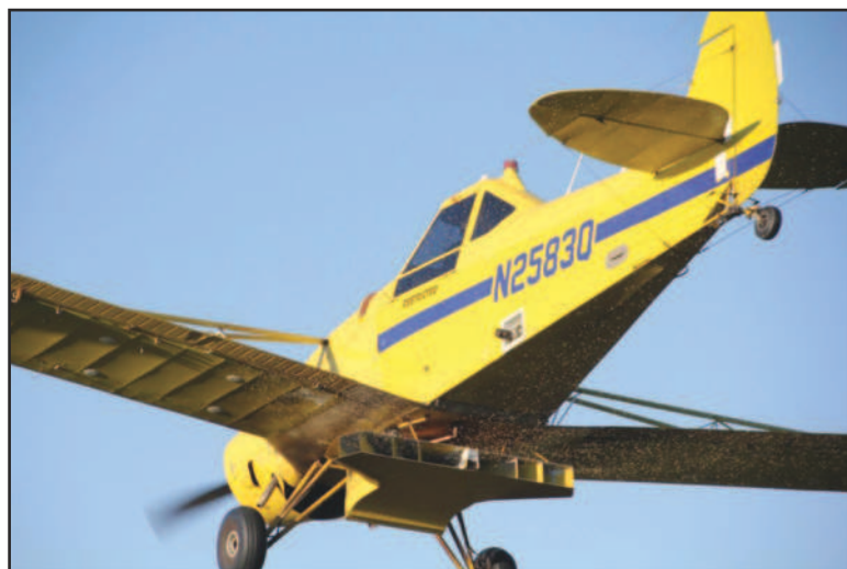
Tony uses a spreader box attached to the bottom of his airplane to broadcast seed.
